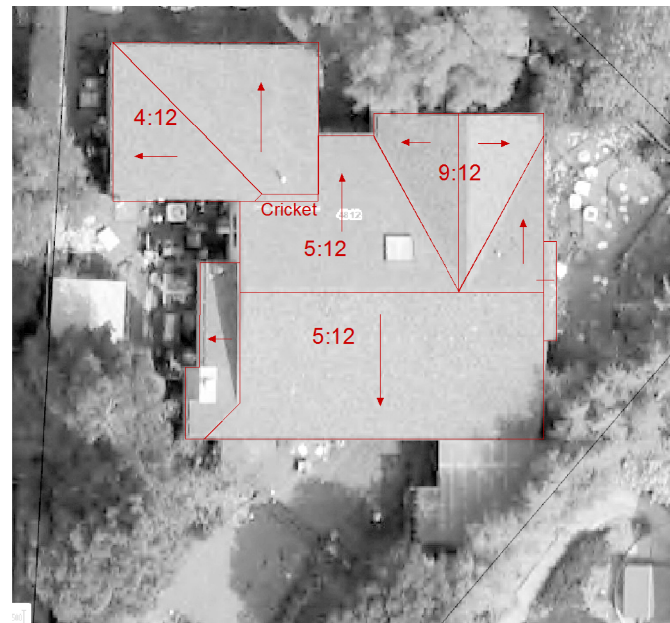
Existing Roof Slopes shown for information
